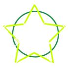
Star Pattern: for sampling from a damaged area.
